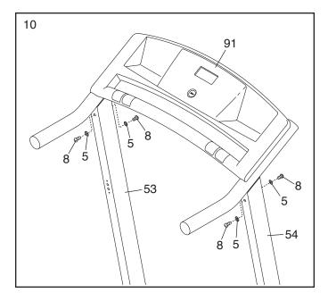
With the help of a second person, carefully lower the Left Upright (not shown) and the Right Upright (54) to the floor.
